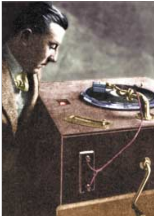
3 A promotional mock-up of the 'Phonovisor'. The image would appear in the aperture to the left of the turntable. A single pickup arm would playback video and audio together in a manner patented by Baird several years before Alan Blumlein's 1931 stereo patent [Courtesy of the author]
